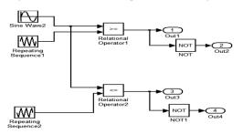
Fig: 6. Circuit Diagram of Pulse Generator
