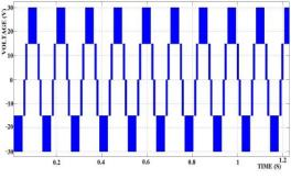
Fig: 7. Five-Level Cascade Multilevel Inverter Output Waveform
