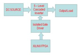
Fig: 1. Block Diagram of Cascade Multilevel Inverter
