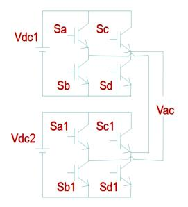
Fig: 2. The cascaded H-bridge multilevel inverter circuit Table: 1. Gate Switching Signal for Cascaded Multilevel Inverter
